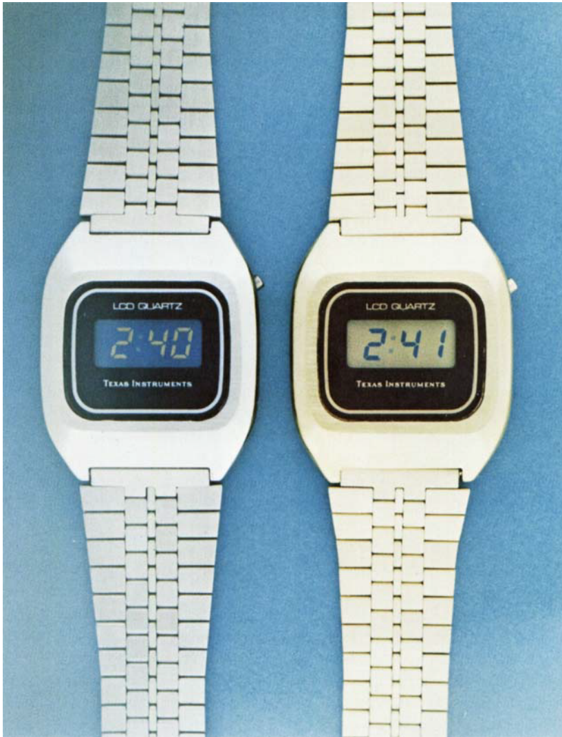
FIGURE 3 Phase Retarder Displays. Operating phase retarder displays are shown in stainless steel and gold cases. On the right hand side the polarizers on the display are crossed as in Figure 2. Blue letters on a gold field results. On the left hand side the polarizers are parallel producing gold letters on a blue field. The blue field is visually very pleasing, but the off axis contrast is inferior as is the case with all parallel polarizer cells. The fidelity of the colors can be judged relative to the familiar colors of the stainless steel and gold cases and bracelets. The optical retardation for both examples was \Delta nd = 1\lambda . The details of the display construction are described in the text.
